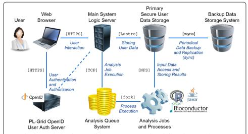
**Fig. 1** This diagram displays the setup of the DNA microarray analysis platform. The main web server performs third-party authentication using PL-Grid OpenID, and subsequently serves authorized content. Large-scale computations are performed asynchronously in a job queue and all user data is backed up to secure secondary storage for additional fault tolerance
