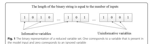
The binary representation of a reduced variable set. One corresponds to a variable that is present in the model input and zero corresponds to an ignored variable.
