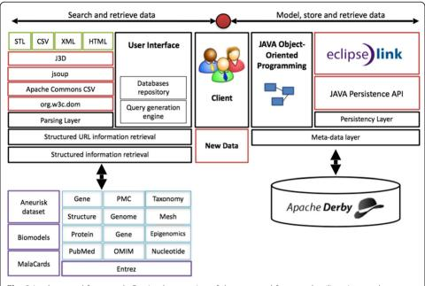
**Fig. 2** Implemented framework. Our implementation of the proposed framework utilizes Java as the development environment, EclipseLink as the JPA provider and Apache Derby as the database manager. Parsing layers were based on J3D, jsoup, Apache Commons and Org.w3c libraries. We implemented structured interfaces to various databases including MalaCards, Biomodels and several NCBI's data sets
