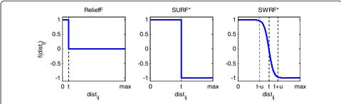
**Figure 1** \*Neighbor weighting functions for ReliefF, SURF\*, and SWRF\*. The x-axis for each plot denotes the distance of sample  $s_j$  from sample  $s_i$  and the y-axis denotes weight in the range [-1, 1]. Parameter t represents the function center and was set to the mean pairwise distance between samples. Parameter u is the function width and was set to the standard deviation of pairwise distances.
